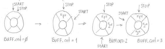
Once the main program is finished with the blocking task, it sees that BUFF-cnt \neq \0, thus gets the scan code as "1" and displays it. Decrementing BUFF-cnt by one does not empty the buffer, so this is repeaded for "2" and "3" Hence
