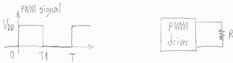
$$\text{Average Power} = \frac{1}{T} \int_0^{T_1} \frac{V_{DD}^2}{R} dt$$
